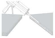
Position the two components to be joined opposite one another with a 3 to 4 mm gap between them. Apply a further bead of adhesive in the joint: this should ensure a seamless joint.
