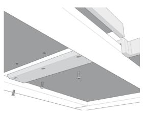
After the pRaL® components have been fitted, the expansion joints need to be sealed
