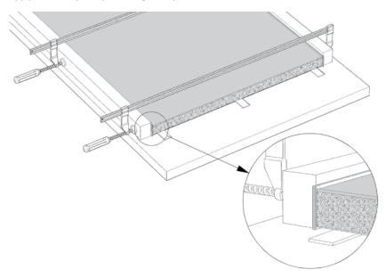
o After the curing of the glue, cut the edge strip to size and sand it.
