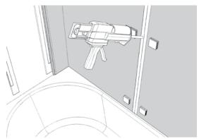
o Next, clamp the two pRaL® wall sections together with jointing clamps using the plywood blocks fastened with hot-melt adhesive.
