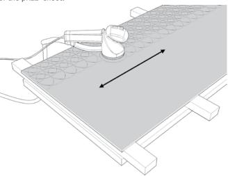
o For final sanding and finishing it is best to use the polishing method: namely a random figure-of-eight action diagonally across the pRaL® sheet, in a smooth, not too abrupt action.
