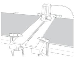
o The butt edge can be cleaned up using a cutter with a top guide bearing plus an MDF or solid plastic guide.
