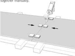
o Clamp the components together tightly with jointing clamps using the previously glued plywood blocks, such that the adhesive is forced out of the joint everywhere. Retain as little adhesive as possible in the joint.
