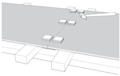
o Grind off surplus cured pRaL® adhesive as close as possible to flush with the surface, using two battens underneath in MDF or solid plastic, of exactly the same thickness, as a guide and a spacer for the top router. Use a copying ring, size 30 mm for instance, between these two battens: this can be a handy aid.
