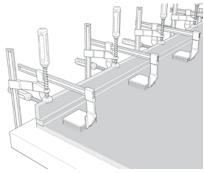
• The clamping arrangement can be released after curing of the glue and the rounded inside corner can be machined with a moisture barrier or barrel cutter.
