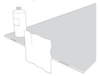
o Ensure that the two pRaL® components to be glued are in perfect horizontal alignment and in the correct position. Also ensure that the pRaL® reinforcing strip can be placed under the glued joint.
