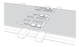
o  $\;$  Apply the pRaL® adhesive to the pRaL® reinforcing strip and position it centrally under the joint.
