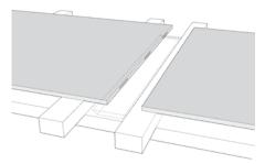
o Apply hot-melt adhesive,  $50 \times 50 \times 18$  to 25 mm thick plywood blocks to the pRaL° components either side of the glued joint. Set the blocks at approximately 300 mm apart and a minimum of 10 mm from the adhesive joint.
