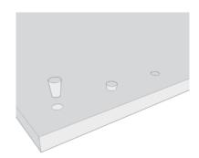
• More substantial damage is to be cut out with a tapered tool and can be repaired by gluing in a fitted pRaL® piece.
