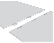
Tip: In case of edges showing rough cutting or milling, sand the two edges to be butt-joined and the surface of the reinforcing strip with 150/180 grit sandpaper.
