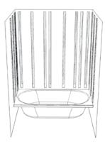
o Start by fitting a corner section. Apply a bead of MS polymer adhesive to the battening
