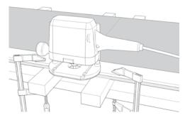
Sand the surface smooth with an orbital sander. The sander should be fitted with a hard sole-plate such that the wave effect when sanding is reduced to a minimum.
