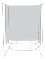
o Apply MS polymer seal horizontally between the horizontal bathroom unit and the vertical pRal® wall as well as between the pRal®wall and the ceiling in order to create a watertight seal.
