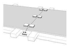
o Fill the joint with the colour-specific pRaL® adhesive and press the pRaL® components together manually.
