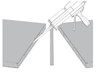
o Apply pRaL® adhesive to the opposite butt edge of the timber substrate, in the form of upper and lower beads of adhesive with a zigzag bead running between them, as well as in the groove opposite for the pRaL® tongue.
