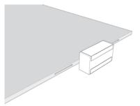
o Ensure there are no pencil lines, imprints or other marks on the pRaL® surfaces to be glued (or in places where the adhesive might exude). The solvent effect of the adhesive will bring the pigmentation of the marks to the surface and make the joint visible.
