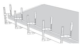
• The jointing clamps can be released after the curing of the glue and the pRaL® glue-line can the be machined flat using a straight cutter with a guide bearing.
