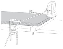
o Cut openings for the sheet jointers on the underside; two of these for a sheet width of 60 cm is sufficient. Cut them to a sufficient depth such that when the glued faces are clamped, the clamping force is greatest on the visible side. Accordingly, it is recommended that the jointing clamps are positioned at or beyond the mid-point across the thickness of the sheet.
