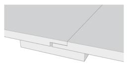
o The reinforcing strips can best be glued in the workshop to one of the two pRaL® wall panels to be joined together.
