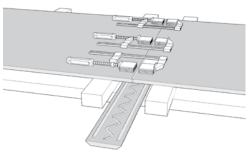
o Clamp the pRaL® reinforcing strip to the workpiece by means of jointing clamps using the previously glued plywood blocks.
