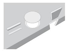
• A pRaL® basin with a visible or split glue-line can be cut free using a special disc cutter and glued back in again (with pRaL® adhesive). NB: this is not a simple operation, it requires both the worktop and the sink to be held perfectly in position.
