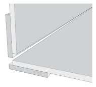
o The two prepared panels will then require to be glued together perfectly square. It is recommended that a jig be made for this which can act at the same time as a structure to transport the corner unit. Also ensure that the inside corner is still accessible in order, once the adhesive has cured to a limited extent (after 15 to 20 min.), to remove most of the adhesive residue with a sharp wood chisel. In this way subsequent sanding work can be reduced to a minimum.
