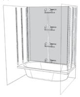
o Keep the pRaL® panel in place by wedging it with planks from an opposite wall or by means of a structure between the floor and the ceiling.
