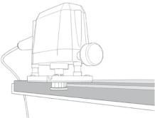
• Sand the pRaL® glue-line smooth with an orbital sander fitted with a hard sole-plate and P280 grit paper, in a rotary action. Take care when sanding smooth to ensure that the pRaL® backsplash is not rounded off.
